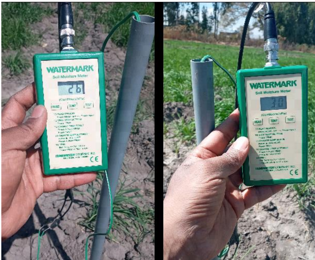
Figure: 5.4: Soil moisture level measuring at field using Watermark
